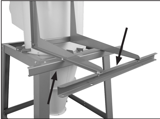
Figure 27. Long brace supports attached.
